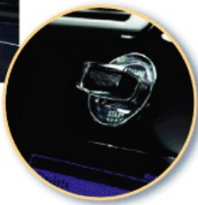
The Aston Martin DBS uses an electronic key fob and mating docking station developed by STRATTEC exclusively for Aston Martin.
